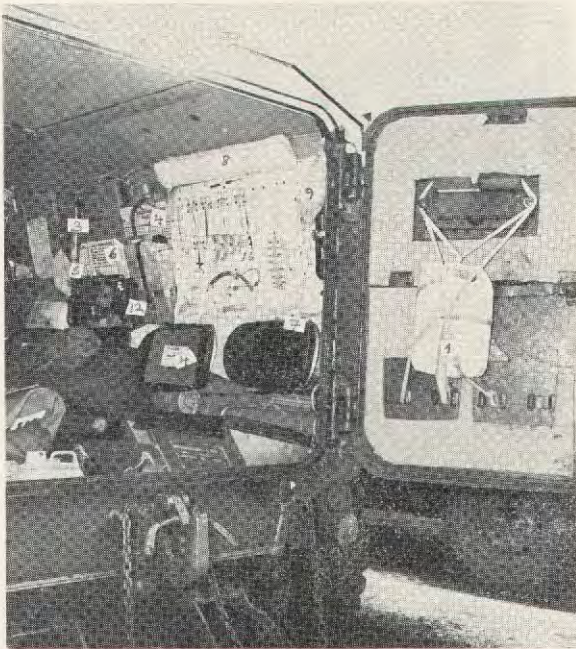
Fig. 1. Burns solution on door (1). Street index above radio (3). List of equipment under seats and tracheostomy set (4). Radio and frequency chart above (5). Noti-cas procedure above radio (6). Shell dressings behind seats (7). Splints (8). Drip fluids (9). Torch (12). Instrument display (16).
