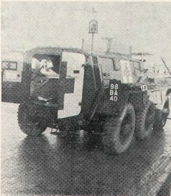
Fig. 4. Saracen ambulance showing extra stretchers (15) carried on the exterior of the vehicle to allow for maximum room inside.
