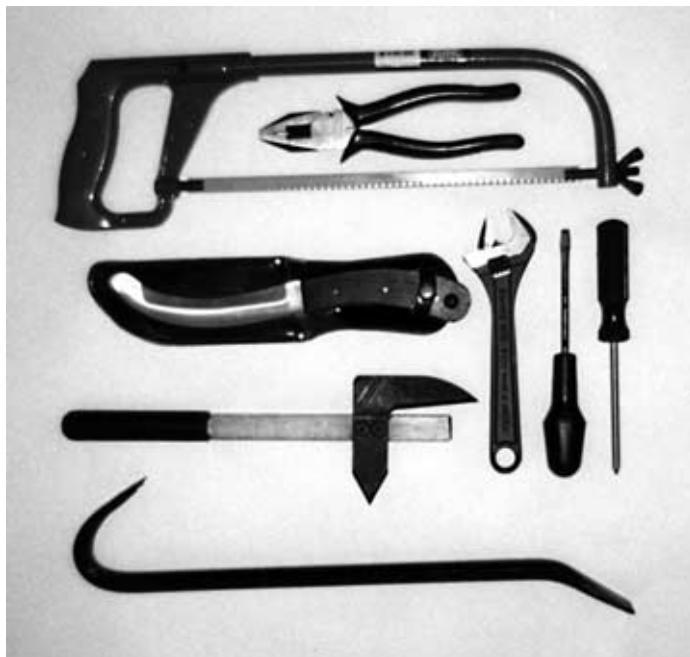
Fig 2. Rescue Tools carried on Military Ambulances Hacksaw, pliers, flatpoint and crosspoint screwdrives, 18 inch wrecking bar (crowbar), 8 inch adjustable spanner, release knife, Keech cutting tool. Not shown are the leather gloves, portable 'DANGER' sign, 18 inch bolt cutters, guideline (7.35 metres) and tool roll.
