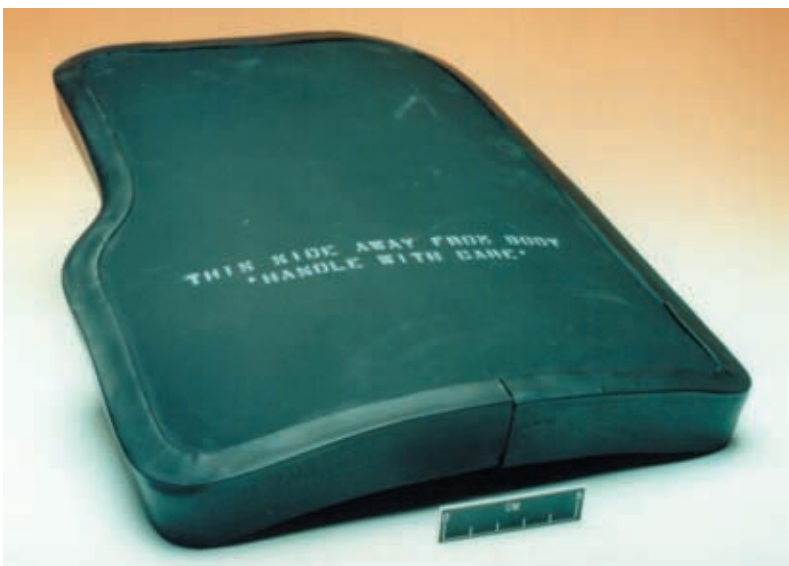
Fig 1. A commercial boron carbide armour plate capable of stopping 12.7 mm bullets.
