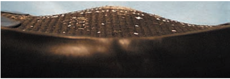
Fig 5. Residual deformation of 20 mm of the rear of a boron carbide plate - the dynamic deformation was greater.
