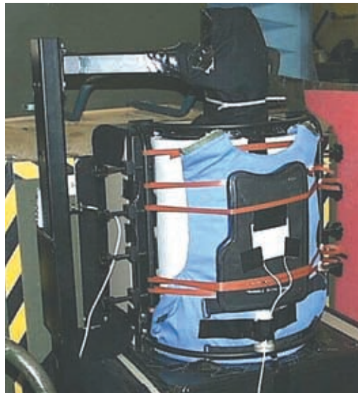
Fig 6. The BABT rig: a boron carbide plate and flexible combat armour system have been placed over the white silicone rubber wall that replicates the dynamic motion of the pig body wall. The rapid deflection of the wall is detected by sequential obstruction of an fan of laser beams behind it (not visible in the image).
