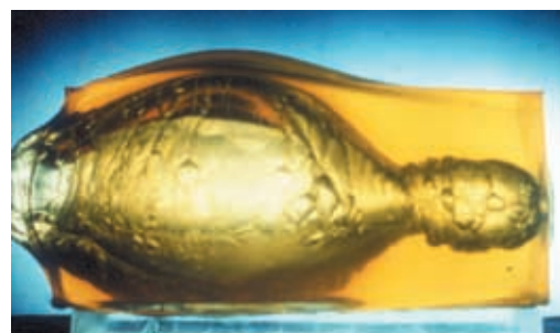
Fig 3. Cavitation in gelatin block from high energy transfer.
