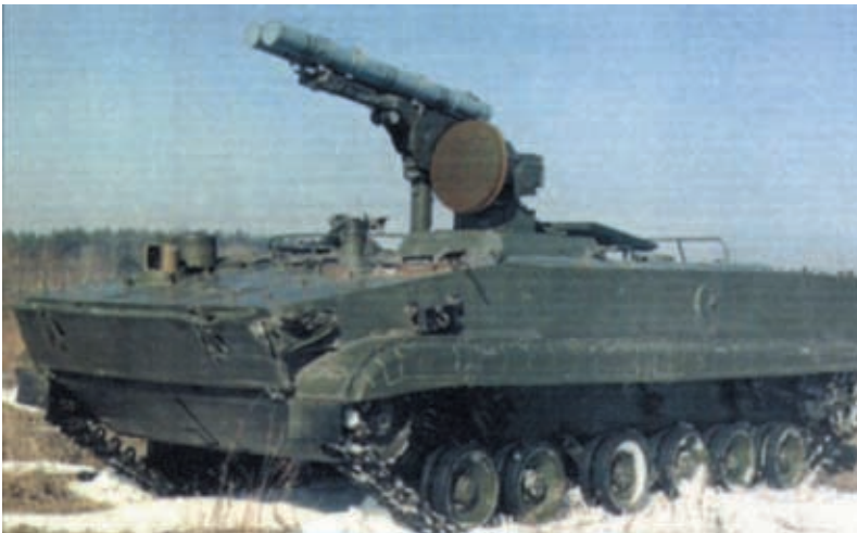
Fig 9. The Khrizantema dual anti-armour/anti-bunker weapon system mounted on a BMP-3 infantry fighting vehicle (1997). Taken from www.geocities.com/area51/capsule/6480/at15htm .
