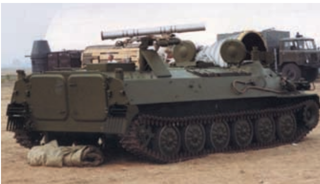
Fig 6. MT-LB tracked vehicle with AT-6 launcher in elevated position (Christopher S Foss).
