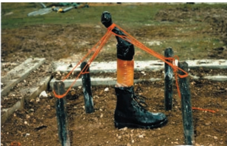
Fig 4. The Lower Limb Model (LLM) used to investigate the failure mechanisms in bone. The bones within the model are from red deer.
