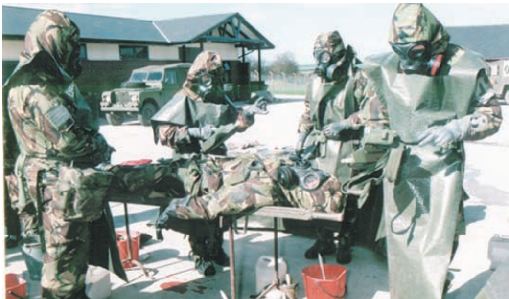
Fig 7. Monitoring contamination on a casualty with the Chemical Agent Monitor (CAM).
