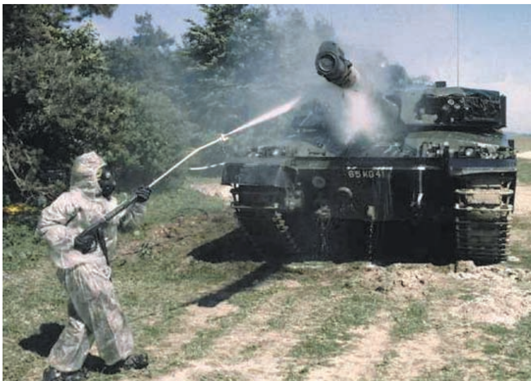
Fig 5. Decontamination of a vehicle with MPDS – Multi-Purpose Decontamination System.
