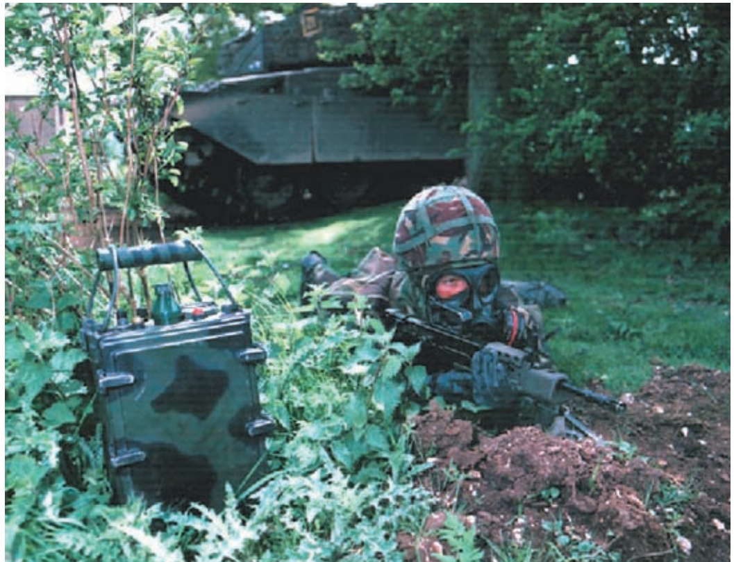
Fig 11. Nerve Agent Immobilised-Enzyme and Detector (NALAD). This was the world's first biologically-based nerve agent detector.
