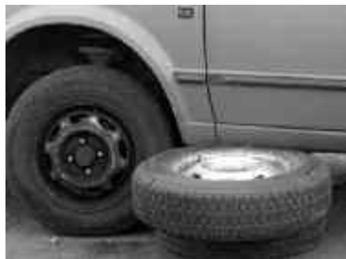
Fig 1. Improvised vehicle chocking.
