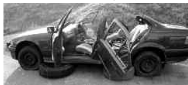
Fig 6. The end-result of a manual-tools-only extrication exercise – achieved within 20 minutes.
