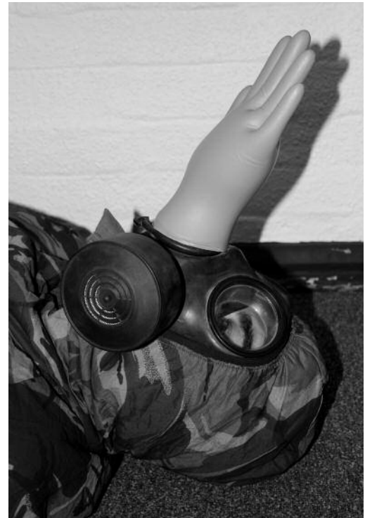
Figure 3. A maximally inflated non-perforated nitrile medical examination glove attached to the primary speech module. The glove became maximally inflated in the first exhalation during the simulation of breathing pattern A (normal breathing).
