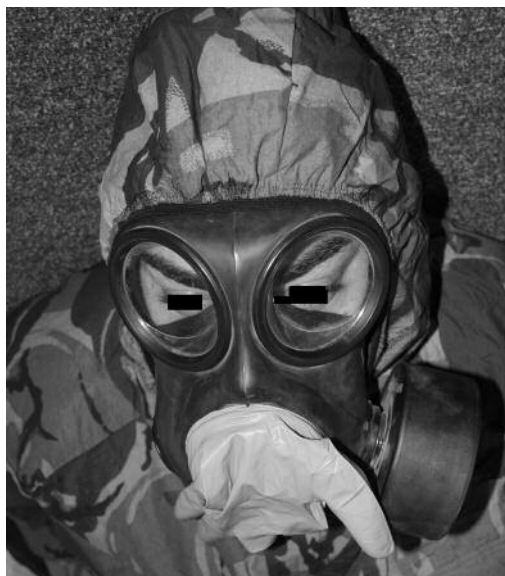
Figure 2. A nitrile non-perforated medical examination glove shown fitted over the primary speech module of the S10 NBC Respirator.
