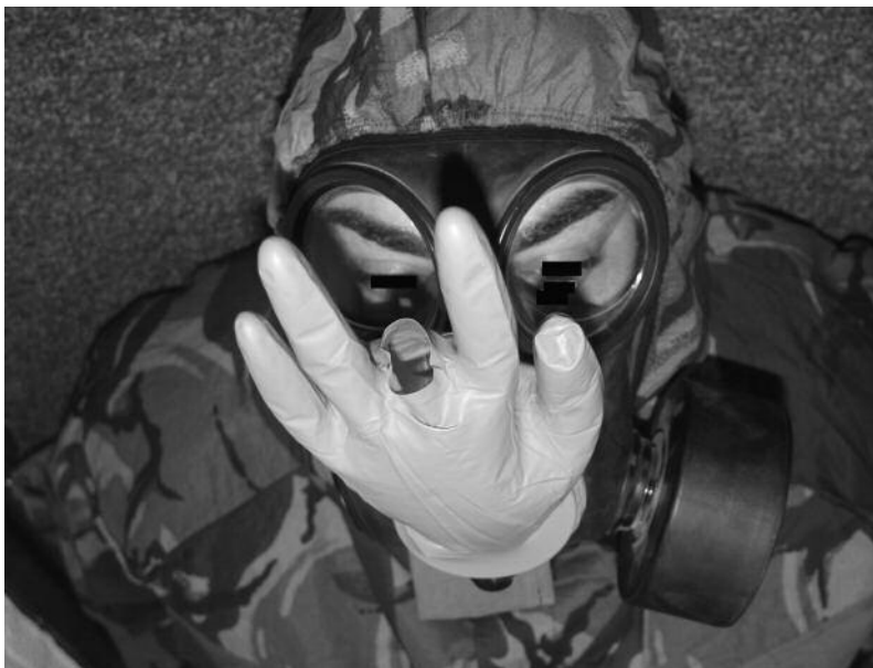
Figure 4. A partially inflated perforated nitrile medical examination glove attached to the primary speech module. The large leak of exhaled air through the hole in the finger prevents the glove becoming fully inflated during this breathing pattern B (hypoventilation) simulation.
