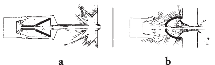
Fig. 2. Diagram showing the principles of the Shaped Charge Missile.
