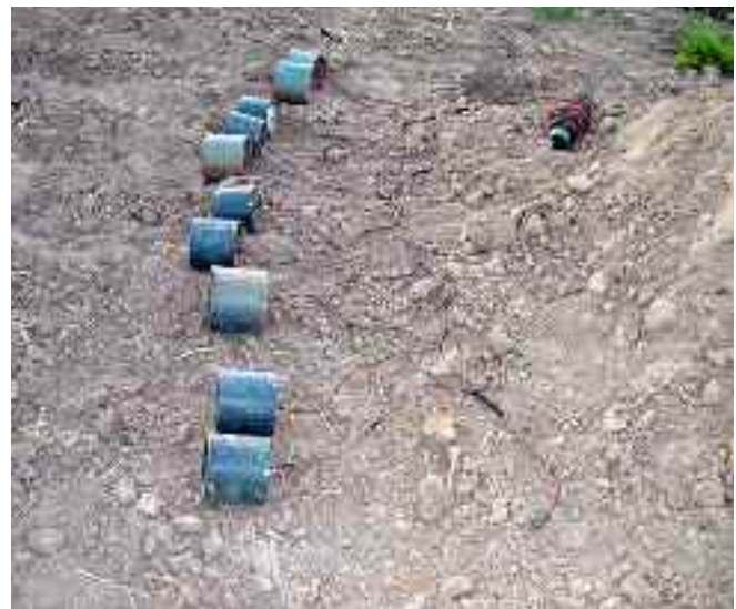
Figure 1. A number of EFPs linked in a daisy chain configuration, uncovered in Iraq. (From: MOD archives with permission. Crown copyright)
