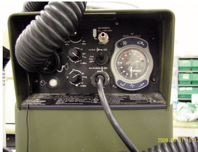
Figure 1. Initial ComPAC 200 ventilator settings for the ventilation of children weighing 10kg or less.
